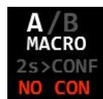
*The green text will show the type of console the Macro Stream SD is communicating with if the configuration and network connection is good. But here the correct license pin isn't entered yet.*
